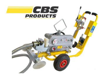
Duct Rod Pushers are designed to assist in rodding operations. The units are mounted on sturdy, anti corrosion treated tubular steel frame, and fitted with gel filled puncture proof tyres, with hydraulic controls mounted on the frame for ease of transportation. The pushers are fitted with a tilting extendable boom, and chamber clamp for use in underground structures.
